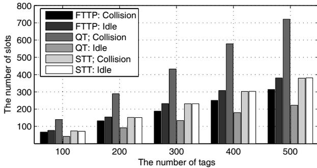
Fig. 4. Collision slots and idle slots consumed to identify all tags.
