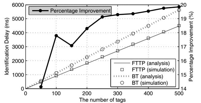
Fig. 3. Identification delay versus the number of tags; comparison of simulation and analysis.
