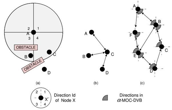
Fig. 2. Network Model and Illustration of  $\alpha$ -MOC-DVB. (a). The network has obstacles. (b). The directed graph of the network. (c). Illustration of  $\alpha$ -MOC-DVB property.
